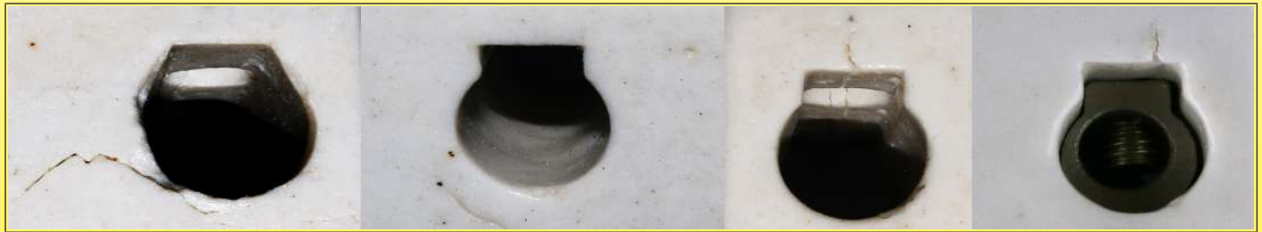
Examples of cracks on C111 porcelain
