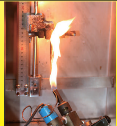
Specimen during UL94VO checking
