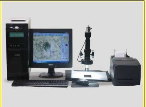
Electronic microscope measurement of the indent diameter (Ultimheat Laboratory)
