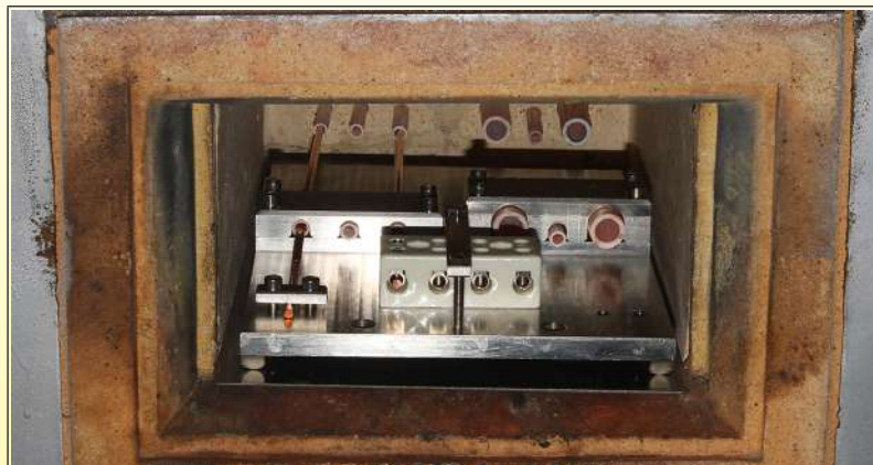
Test oven for the resistivity of ceramics as a function of temperature (Ultimheat Laboratory)
